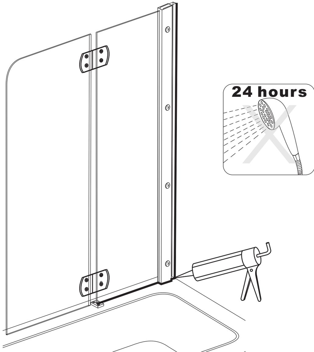
Warning: Don't use the shower enclosure until after at least 24 hours, so that the silica gel can be totally dry.
